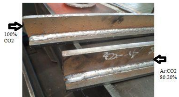
Fig-9 Welding Spatter
